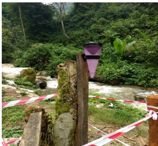
Rain gauge installed by MWE at the site
